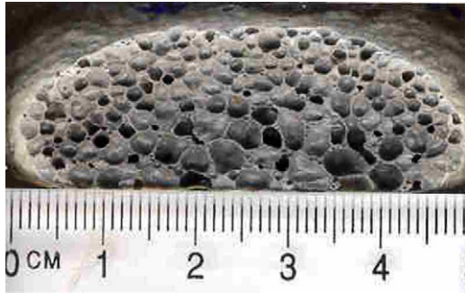
Fig. 8. Microstructure of the sample with 6% abrasive addition in the polishing residue after sintering (digital camera).
