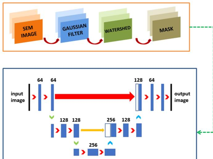
Fig. 1. The workflow of pre-processing of SEM images as input data and Neural Network (Unet) for computational simulations.
