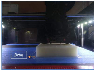
Figure 11. Object being printed using Brim.
