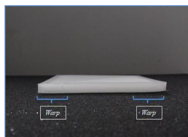
Figure 10. First attempt to print the accessory to couple the dosimeters, showing a warp on the sides of the piece.
