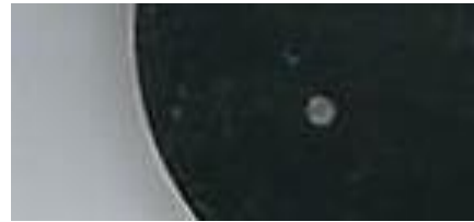
Figure 4. Example of wear crater obtained.
