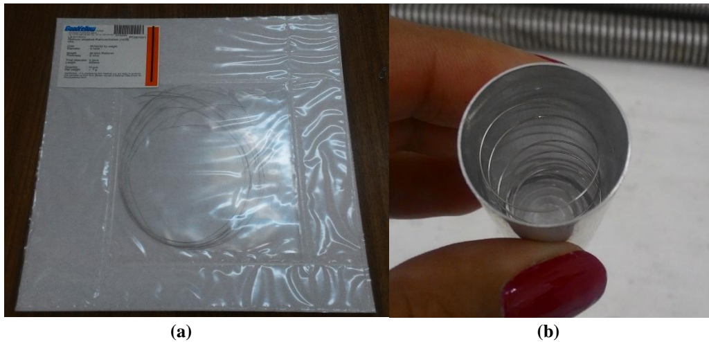
FIGURE 3: a) Wire before irradiation; b) Twisted wire inside irradiation tube.
