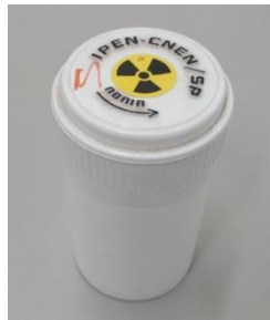
FIGURE 5: Shielding and storage device. Dimensions: 10 cm height and 5.2 cm diameter. Volume = 212.37 \text{cm}^3 .
