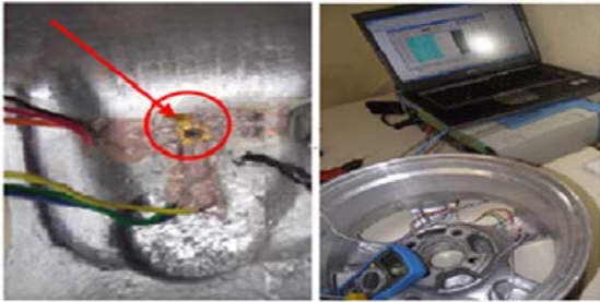
Figure 3: Hole drilling method experimental sequence of trial.
