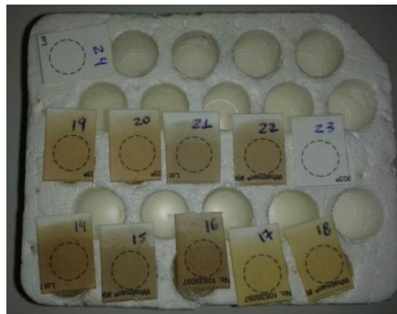
Fig. 2. Deposition of samples paper substrate using polystyrene as a support.
