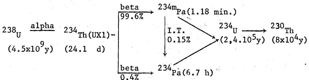
Protactinium-234m (1.18 min.) as a short radioisotope has great interest for radiochemistry experiments (1-6) and for dead-time determination (6,7). Since it is a reasonable short lived
