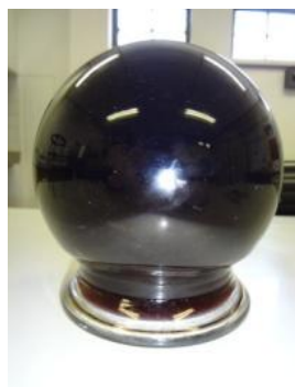
Fig. 2. Spherical glass balloon filled with FXG solution: the head FXG phantom without human bone.
