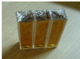
Fig. 1. PMMA cuvettes set filled with FXG solution.
